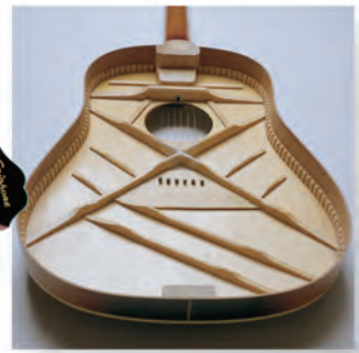
Traditional X-bracing and careful kerfing make the top sing
